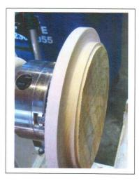
6) Put second blank in chuck and use to make a tight fitting jamb chuck. Frisbee should be snug. Too tight can crack it.
