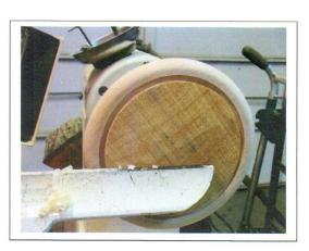
Using a parting tool, create clear bottom edge. Also use parting tool and depth gage to set maximum depth to establish thickness of Frisbee.
