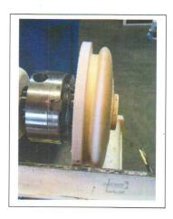
7) Make jamb chuck so fingers can get behind Frisbee to pull when completed.
