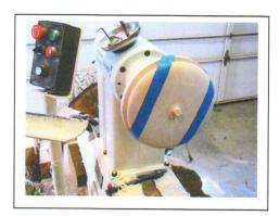
8) Tail stock can be used or blue painter's tape applied to increase stability while on jamb chuck.
