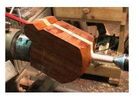
After turning the spout I take the piece back to the bandsaw and trim off some of the excess on both sides of the handle.
