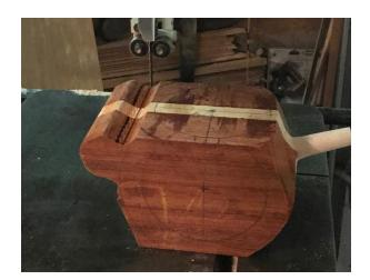
This next step is not necessary but I find it useful to create a reference for maintaining an area for the bottom recess while rounding the sides. I drill a hole in the top and mount the piece in the four jaw chuck using a worm screw. I then partially round the bottom to locate the outside diameter of the mounting recess.
