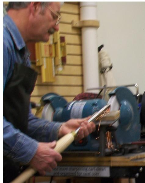
Liam uses 2 bowl grinds: long side grind and a regular grind;
