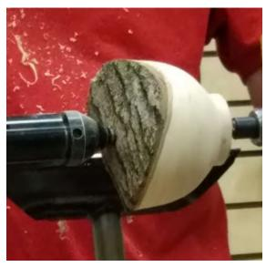
The outside is finished, and chuck tenon has been formed.
