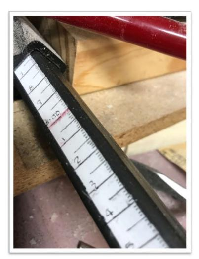
PS: I originally thought of taping a metric scale on the arm. This would have been less tedious and more accurate, but the tolerance between the arm and the square hole is too tight. Therefore, the white paint seemed like an easy solution.
