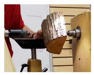
**MOUNTED PERPENDICULAR TO THE LATHE BED**
