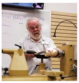
NOTE THAT THE WORK PIECE IS MOUNTED WITH GRAIN
