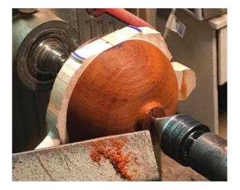
Despite creating a reference for the bottom, I ended up cutting in to the area that I had planned on leaving for the bottom recess. The reference simply kept me from going even farther and ruining the blank. After turning both sides, I remounted the piece using a worm screw, and adjusted the bottom, turned a recess, and shaped the bottom up to my side mounting points.
