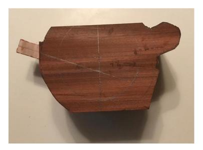
I then mount the teapot between centers and turn the mounting tenon for drilling and turning the spout.
