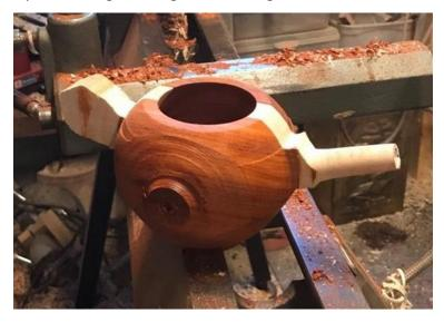
After completing turning on the lathe, I use a marker to finalize the basic shape of the handle. I also use a circle template to locate and define an outline of the feet on the bottom rim around the recess that I turned for chucking.
