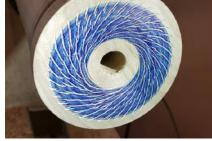
Here I used the same mini-tool set it at a slight angle, about one o'clock position, then moved the tool to the left while I continued to rotate the tool to about a two o'clock position near the edge. Again, it was colored and highlighted for a better picture.
