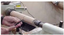
Part deeper into the skinny part (not all the way) but will eventually be 1/4" diameter and blend in the taper with a spindle roughing gouge or a regular spindle gouge.
