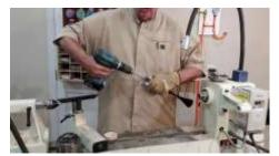
Drill a hole in the bottom with a 1" drill bit using a jig to hold it steady. Or use your hands to hold it steady.
