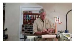
Then put a tenon on one end, mount in a 4 jaw chuck.
