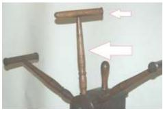
Walt Connerm. my first-ever project, I have pointed at the replacement spindle for a friend's yarn winder, 13" long and 1 1/4" in diameter
