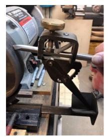
Measure and cut a piece of Masonite or plywood to tightly fit the gap as shown.
