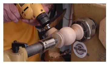
Two hemispheres glued together and final sanding in progress.
