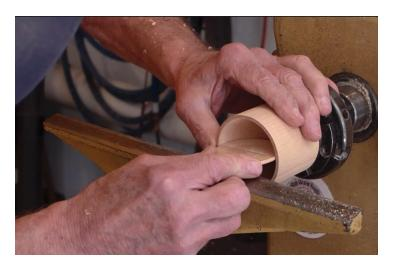
The internal sphere is perfect when the diameter line of the circle gauge exactly matches the edge of the work piece and there are no gaps or humps on the inside.
