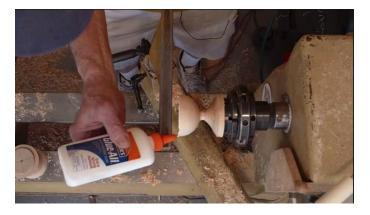
This is a complete hemisphere, ready for gluing to another hemisphere. Wall thickness is  $1/16'' \pm ...$
