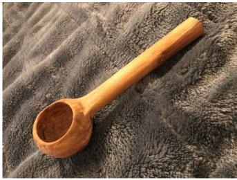
From Brad Miller: Coffee Scoop 6" x 1.75", made from Bradford pear and finished with Danish oil. He used multi axis turning to get a deep scoop, then mounted bowl in turned jig to hollow the bowl. The bottom is flattened to stand up without spilling.
