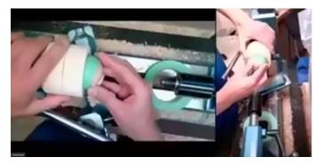
Next, wrap the salt cellar blank with masking tape to keep the wood from being bruised by the jamb chuck body and to aid in the fit. Then insert the spout in the jamb chuck drilled hole
