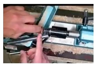
Make the button (hole plug) first and then turn the hole to suit.
