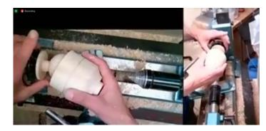
Testing the fit of the jamb chuck with the spout in the drilled hole.
