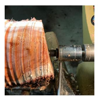
The next challenge is to accurately and securely screw the faceplate to the workpiece. My faceplate is threaded straight through so I measured the opening.
