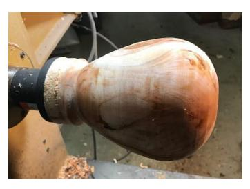
I left sacrificial wood at the base to allow for screws and final shaping of the bottom.
