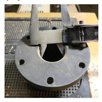
While the piece is still mounted between centers, turn a stub to fit the opening of the faceplate. Make a large enough flat to safely accept the mounting screws.
