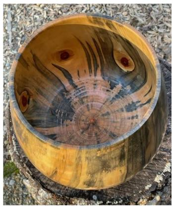
This is Norfolk Island pine (NIP), finished with 3 generous coats of Minwax Antique Oil. When dry, NIP is very porous and soaks up the finish. If turned to a thin wall, it will become translucent. The wall thickness is about 3/16ths", height 7 ½" and width 8".
