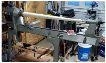
My steady rest is not large enough for the Nova lathe and I had to raise it up by using a piece of plywood as a riser block. It still couldn't support the thinner end. At that point, I could sand the cones using this configuration but not turn them. So, in conclusion, the first one is not done as well as I would like. The second one came out looking much better.
