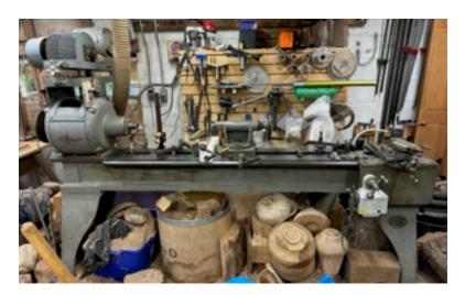
Yates American lathe. 16" swing inboard and 5-6' outboard. Between head and tail stock is almost 6 feet. Plenty of room for most architectural spindle turning and/or large bowls/platters.
