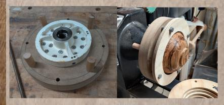
A 6" face plate (heavy duty FP is best) is mounted to a 10" diameter plate. In the version I have which came from Alton Bradford, 4 3/8" diameter bolts are used to attach the doughnut ring (which is placed over the bowl) to the mounting plate. The rings I have for the 10" mounting plate have hole diameters ranging from 3" to 6.5". For even larger bowls or hollow forms I bolt a larger plate (17" diameter) to the mounting plate which allows me to mount much larger pieces as shown below.
