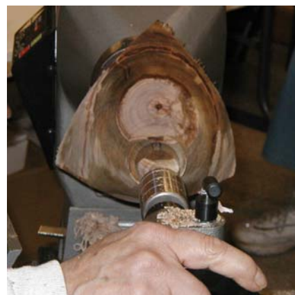
Reversed and Pressed Against the Chuck for Bottom Finishing
