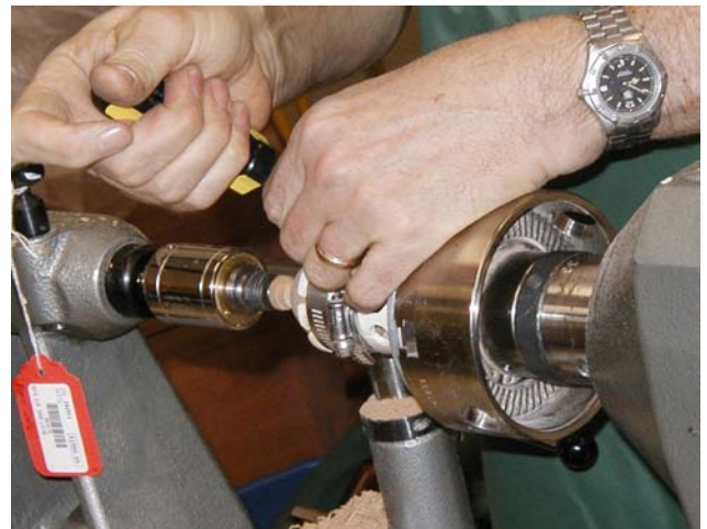
Jig Made of Plastic Pipe For Mounting the Egg for Finishing
