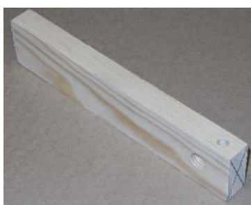
Launch Handle Center Marked and Predrilled for Shaft and String Clearance Slot
