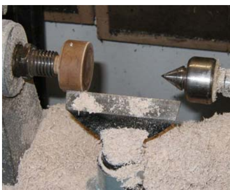
Setup Using a Waste Block with Morse Taper
