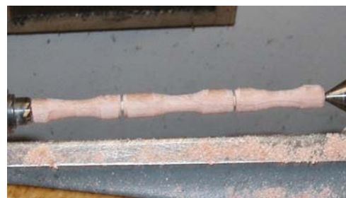
String Pulls Turned Between Centers and Partially Parted
