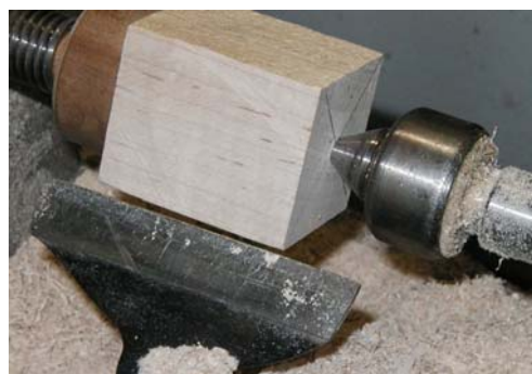
Predrilled Block Compression Mounted Between Live Center & Waste Block
