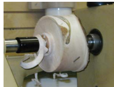
Turn a spigot for chucking.
