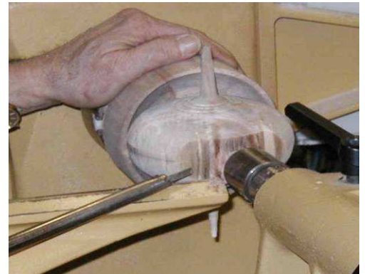
Drilling the hole, 90 degree to spikes
