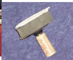
Little something Phil made. Sanding disk that fits into a Nova 2 chuck. Phil provided these photos Thanks
