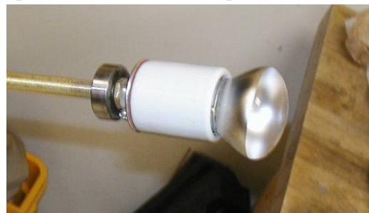
Jam chuck brass tube, bearing & light
