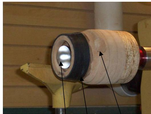
Jam Chuck with light, gasket, & air scoops
