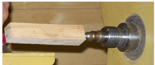
Fan pull drilled blank mounted on lath
