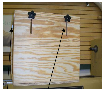
See the adjustable top & reinforcing aluminum angles
