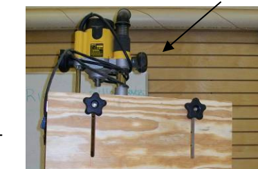
Top with adjustable circle and router hole. Router guide bar. Router setup.
