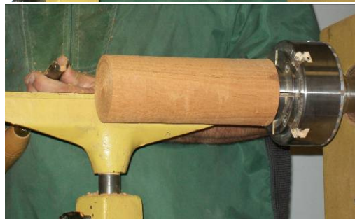
Rough out the outside
