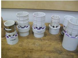
A template of a real egg will help you get started. A 2 X 2 X 3" block makes a nice Grade A egg. Round up the block, mark the center & ends. Remove the excess on both ends and with a parting tool cut down to the diameter of the center of your egg (must be a close fit to your chuck). Shape & sand the egg as much as possible on the lathe. Mount the egg into the egg chuck and turn & sand the ends. Dick Sing has a good book on ornaments & eggs.
