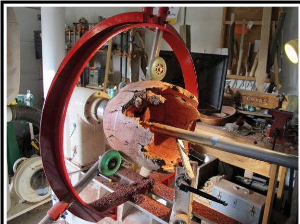
Large manzanita burl being hollowed using large boring bar made by member Alan Weber and being held by Clarke steady rest. The burl was purchased at Woodcraft Jim Bumpas
