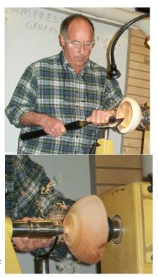
turning the lathe by hand and with a sharp gouge cut off the rest of nub. This will avoid tear out and a flying bowl after you spend all that time making the perfect shape.
