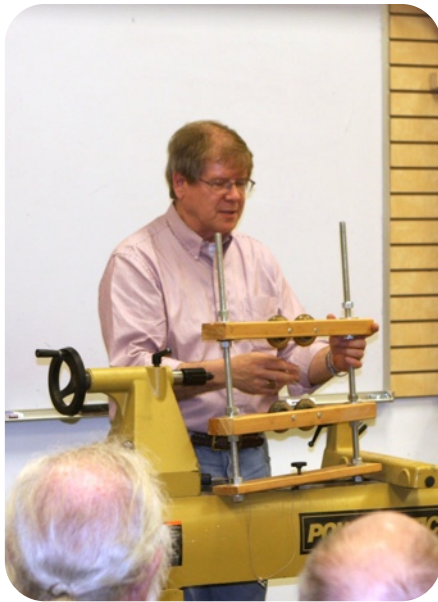
Aage's home made bowl/ spindle steady.
