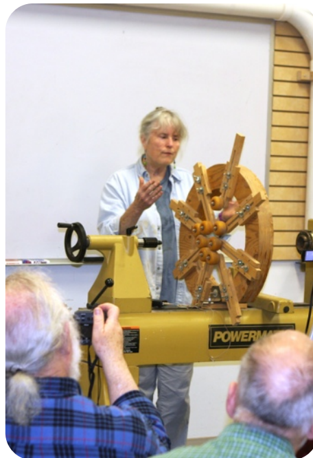
Barbara's home made steady rest (notice the number of stabilizing wheels)
