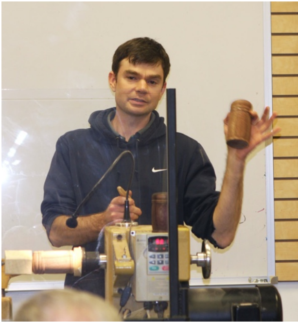
Matt demonstrated texturing a walnut box with a small hand gouge. Using a 2mm U-shaped gouge, small grooves were carved into a thatch-like pattern.
