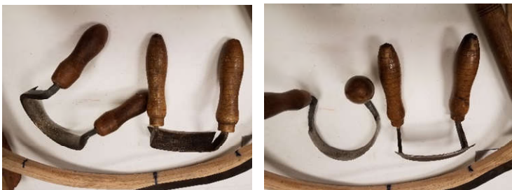
TWO VIEWS OF TWO SCORPS USED TO CARVE SADDLE IN THE SEAT
