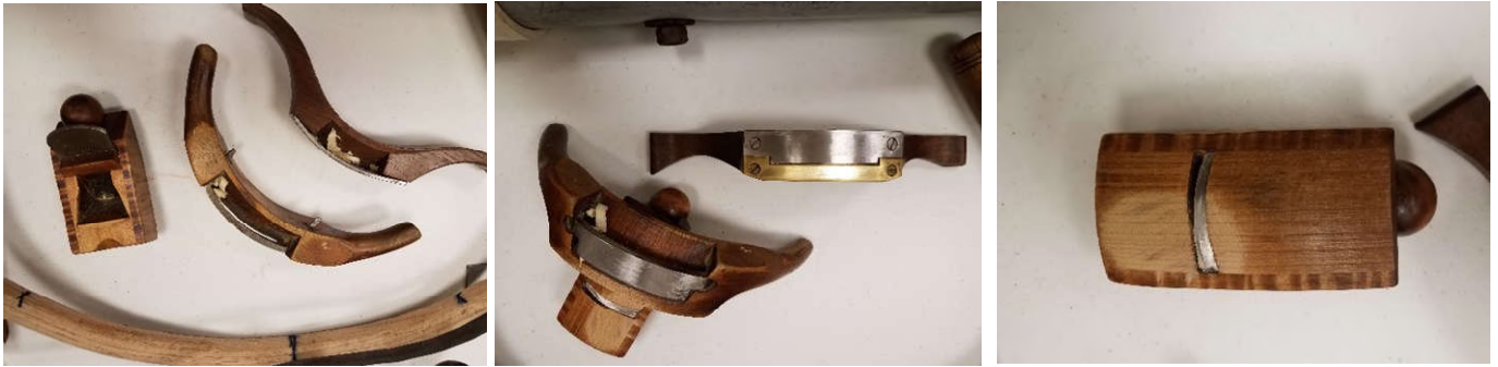
TWO VIEWS OF TWO TRAVISHERS AND A SMALL COMPASS PLANE (CURVED FRONT TO BACK AND SIDE TO SIDE)
