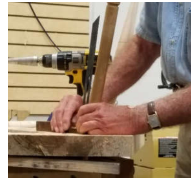
SETTING THE 1 ST LEG IN PLACE, IN THE BACKGROUND IS THE DRILL WITH BIT TO TAPER LEG HOLES.
