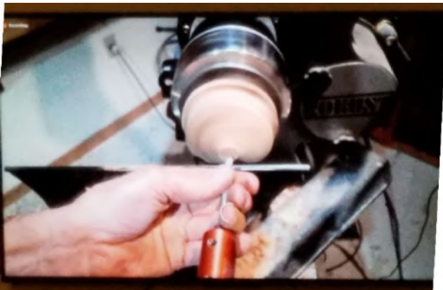
THE CAP TO BE INSERTED THROUGH THE CROWN IS BEING DRILLED TO HOLD A BALLOON.
