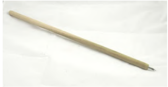
Dan Luttrell, jig for finding center thru tail
