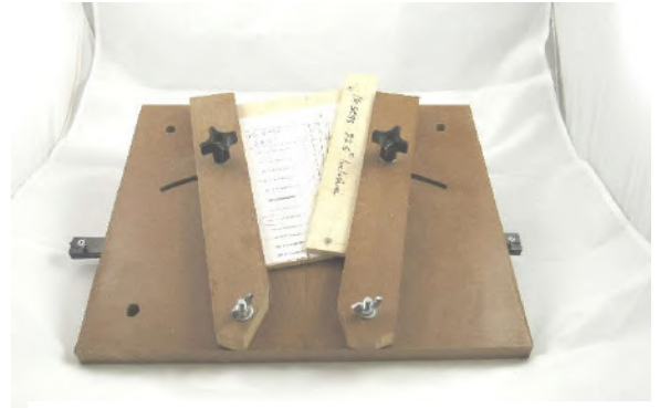
Bill Buchanan, table saw jig for cutting segments
