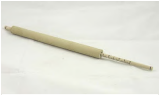
Alan Harrell?, Jig for measuring full length of chair stretcher, inside of mortise to inside of other mortise
