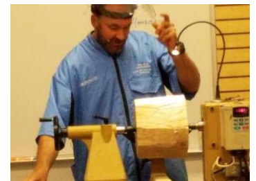
Mounted and ready to start to make it into a cylinder
