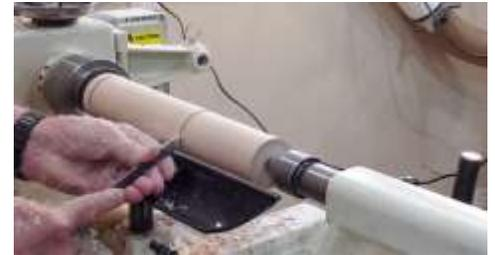
Part deeper into the skinny part (not all the way) but will eventually be 1/4" diameter and blend in the taper with a spindle roughing gouge or a regular spindle gouge.
