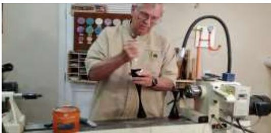
Fill the hole with some sort of weight. I use shotgun shell pellets, even fishing weights will work. Fill with CA glue (or whatever).
