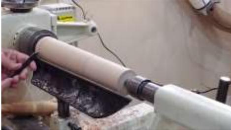
Mark out the waste at the chuck end, with a parting tool mark out the diameter of the top (2") and the bottom (2.5"), and mark 1/3 from the top.
