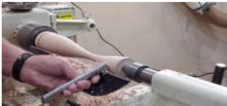
Blend in the top & bottom tapers. I make a set of 12", 10", 8" tall. Sand to #600, I made this set black with shoe polish and spray lacquer.
