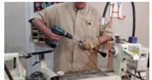
Drill a hole in the bottom with a 1" drill bit using a jig to hold it steady. Or use your hands to hold it steady.
