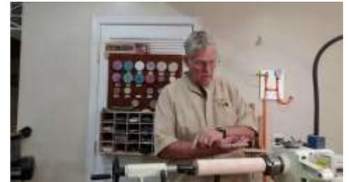
Then put a tenon on one end, mount in a 4 jaw chuck.
