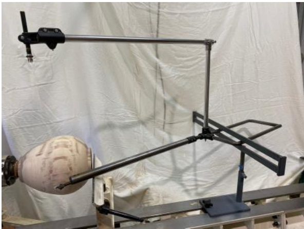
Jamieson Hollowing Rig, As Set Up and in Use
