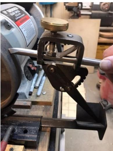
Measure and cut a piece of Masonite or plywood to tightly fit the gap as shown.
