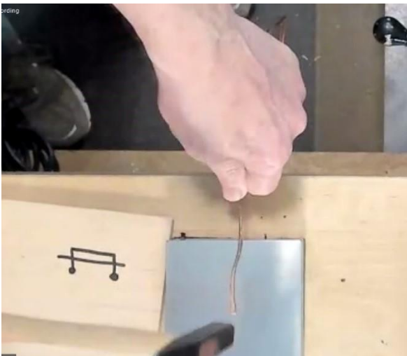
Make staples with 12 or 14 gauge copper wire. Be sure to use a hard and smooth surface to get smooth staples.
