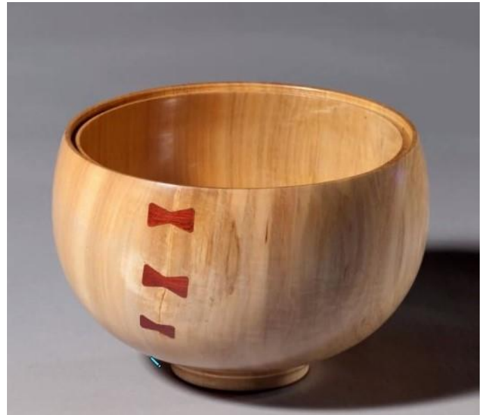
Use inlays for crack repair or decoration. These inlays were tapered in size for effect. In some work, one might want to use all the same size. Check out Big Island Engraving on the internet for kits and instructions. Dennis also offered kits for sale.
