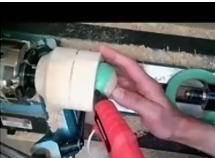
When satisfied with the fit, hot melt glue the workpiece in place. The masking tape will aid in glue removal later.
