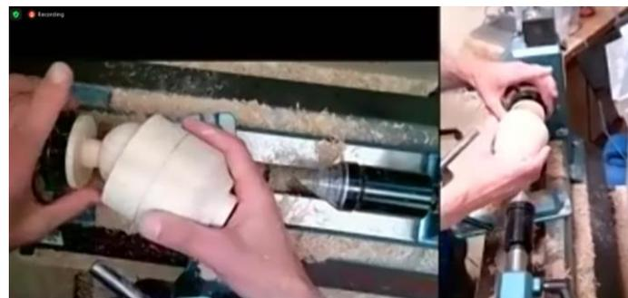
Testing the fit of the jamb chuck with the spout in the drilled hole.
