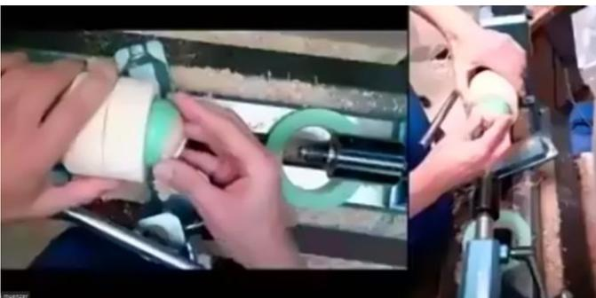
Next, wrap the salt cellar blank with masking tape to keep the wood from being bruised by the jamb chuck body and to aid in the fit. Then insert the spout in the jamb chuck drilled hole
