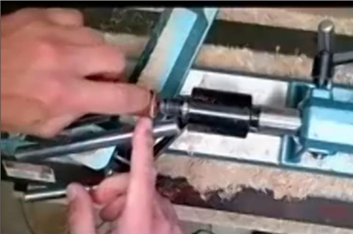
Make the button (hole plug) first and then turn the hole to suit.
