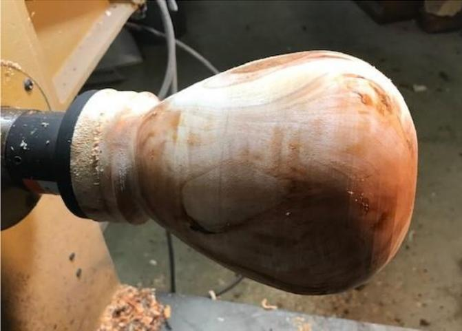
I left sacrificial wood at the base to allow for screws and final shaping of the bottom.
